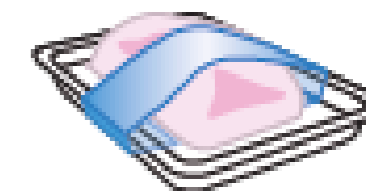
Protruding up to 70mm above height of tray
